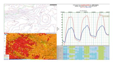
**Fig. 1** Overview of UTCI forecast outputs generated by the Czech Hydrometeorological Institute. Left: fields of maximum (red lines) and minimum (blue lines) UTCI values at 6 h interval, UTCI mapped distribution over the Czech Republic (bottom). Right: meteogram of UTCI and T<sub>mrt</sub> at Teplice (50.51° N, 13.84° E, 236 m asl, top), table of UTCI values predicted at different Czech locations (72-h lead time, bottom). Outputs are visualised via IBL Visual Weather
