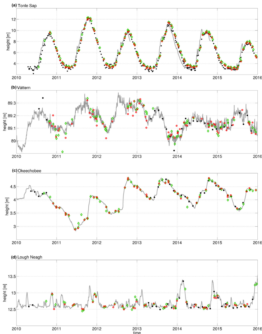
Fig. 6. Water level time series solutions for the lakes (a) Tonle Sap, (b) Vättern, (c) Okeechobee and (d) Lough Neagh: DGFI-TUM (red), gauging stations (grey), DAHITI (black) and DTU (green) (from Göttl et al., 2016).
