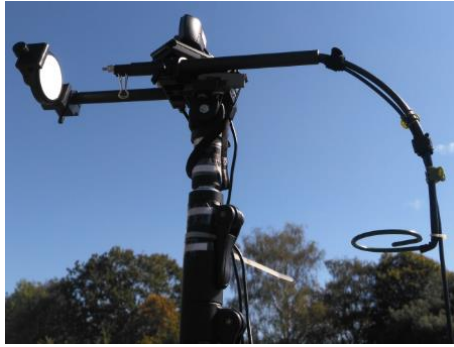
Figure 2. (a) A scalable tripod holding the optical fiber spectrometer for field tests; (b) Optic fiber tip of the spectrometer and a reflectance standard RS50.
