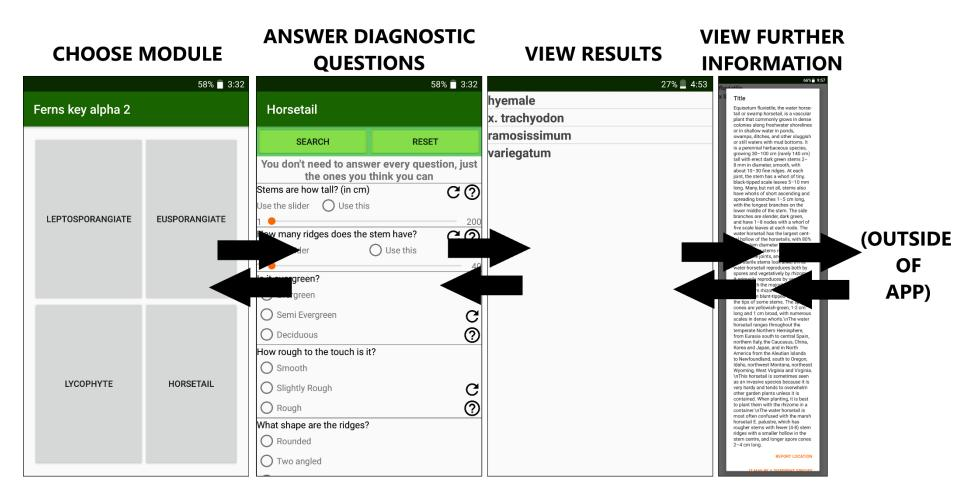
Figure 5-21 – Storyboard for the app as designed. Diagram designed as a hybrid windows navigation diagram and windows layout diagram. Note this diagram shows the use of a single search page; the user can select any of the four options in the 'choose module' window, and will be shown a similar set of windows. Note that this diagram is simplified, with pop-out windows not shown. For a complete windows navigation diagram for this module, see Figure 5-22.
