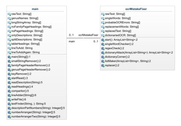
Figure 3-3 - Class diagram of the automatic text extraction program. Note that numbers after ':' refer to numbered points in the method, where the behaviour is explained. Class diagram made using GenMyModel (GenMyModel, 2019) and modified on InkScape (2019).
