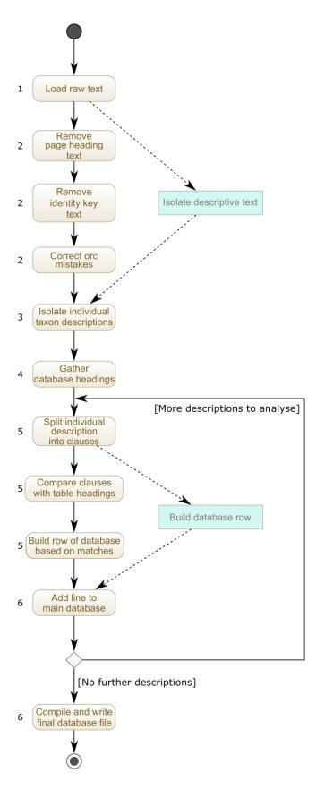
Figure 3-4 - Activity diagram of the data-extraction program. Note that numbers to the left of each step refer to the steps in the method, where the behaviour is expanded on. Activity diagram made using GenMyModel (GenMyModel, 2019) and modified on InkScape (2019).
