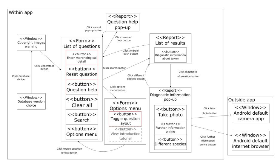
Figure 7-9 – Windows navigation after updates to the app based on feedback. Note that red outlines mean the item is repeated as required for the design and isn't shown here, grey dashed outlines show items that are in the version of the app in Appendix A, but would be in an alternative location in a published version of the app.
