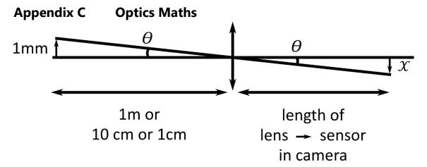
Appendix figure C-1 - Optical diagram, showing an object of 1mm at a distance of 1m, 10cm, and 1cm. The object is to the left of the figure, the image is to the right of the figure.
