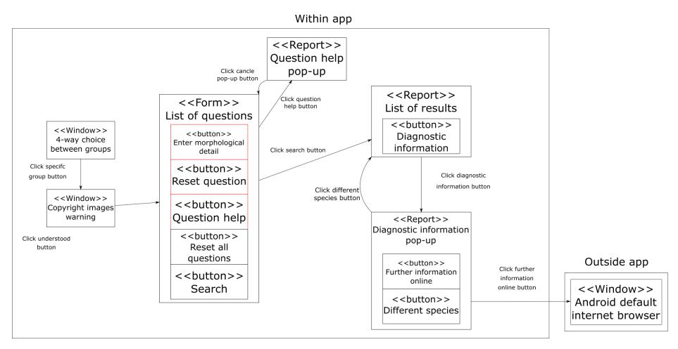
Figure 5-22 - Windows navigation diagram for a single module of the app as initially designed. Note that the set of windows available to the user would be the same regardless of which option is chosen in the '4-way choice' window. Note that buttons with red outlines are repeated as often as required to show all buttons in the form, they have intentionally only been shown once to ensure the diagram can fit on a single page.
