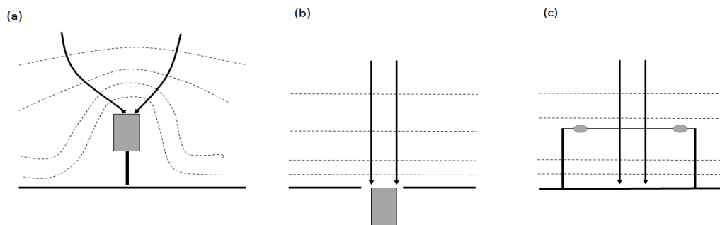
Fig 15.13. (a) Distortion of the electric field (solid lines, with dashed lines showing equipotentials) for a measuring instrument mounted on a vertical mast. (b) Removal of the electric field distortion by burying the instrument in the ground, with its sensing aperture flush with the ground. (c) A passive wire potential measurement is negligibly affected by the distortion effects. (From [15.84])
