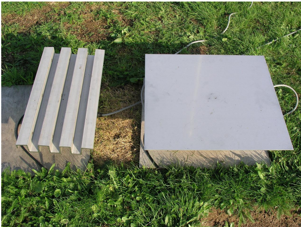
Fig 15.9. Measurement of the conduction and displacement current densities using the combined two electrodes of different geometry in a GDACCS instrument. (Photo: A.J. Bennett).
