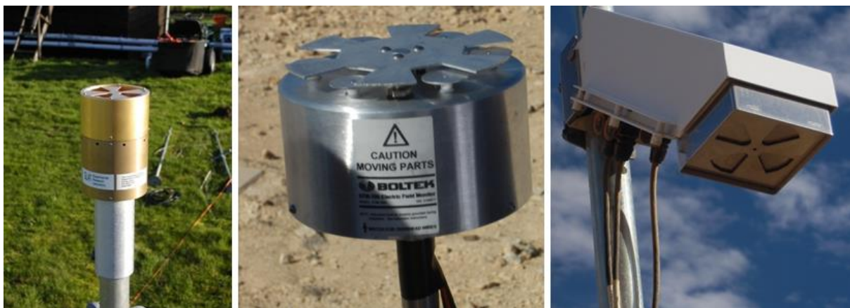
Fig 15.10. Designs of electric field mill: (left) Chilworth JCI131, (centre) Boltek EFM100, (right) Campbell CS110 (Photos: R.G. Harrison)
