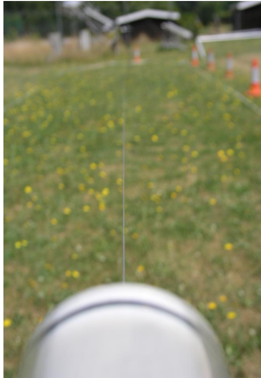
Fig 15.5. Passive wire apparatus showing the thin and long sensing wire emerging from a PTFE insulator. (Photo: A.J. Bennett).
