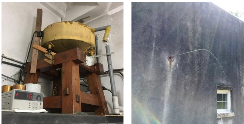
Fig 15.1. Potential Gradient measurements made using the Kelvin water dropper potential equaliser, at Kakioka Observatory, Japan. (Left) Isolated water dropper header tank, with electrometer measuring tank potential. (Right) Water dropper spray, generator from an isolated tube emerging from the observatory wall. (Photo: R.G. Harrison)
