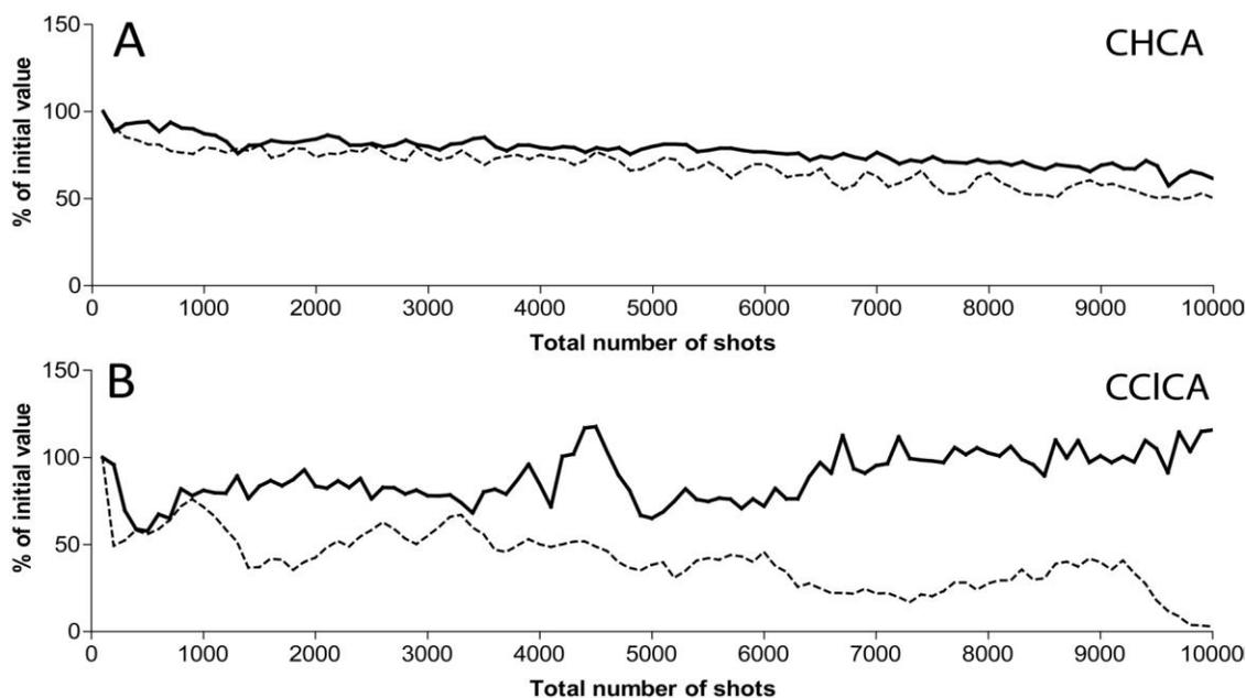
Figure 3. Ion signal intensity of the  $[M+H]^+$  of Angiotensin I with an increasing number of laser pulses. Spectra were acquired as the sum of 100 single-shot spectra at 50 Hz from a single desorption position with  $\sim 1$  sec between each accumulation, for a total of 10,000 laser pulses. Panel A, CHCA-containing LSM (solid line), CHCA-containing ILM (dotted line). Panel B, CICCA-containing LSM (solid line), CICCA-containing ILM (dotted line).
