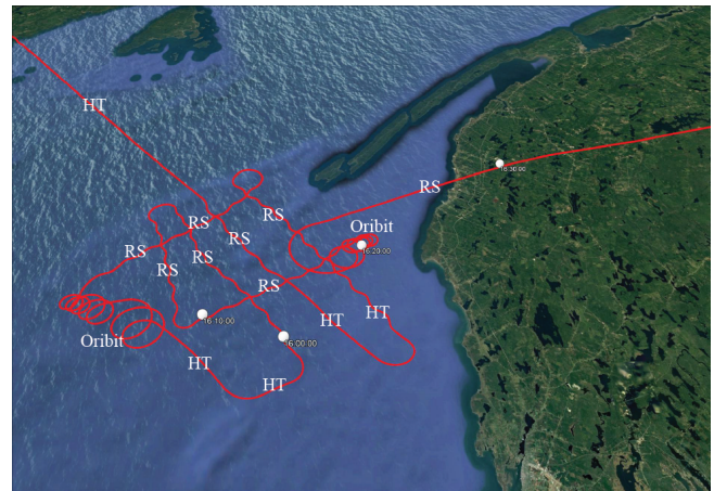
Figure 4. Typical PDPP flight track showing where the aircraft performed a series of horizontal transects (HT), roll sweeps (RS) and orbits of various roll angles.
