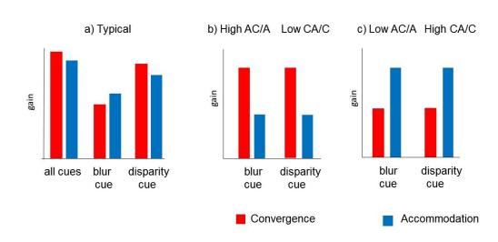
Figure 2. a) Typical response scenario to blur vs disparity cues in relation to all-cue naturalistic responses. b) high AC/A and low CA/C pattern c) low AC/A and high CA/C pattern.
