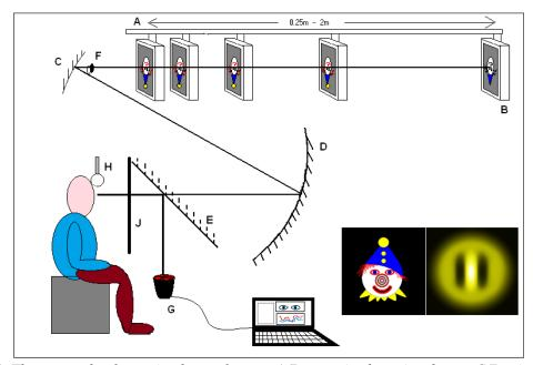
Figure 1. The remote haploscopic photorefractor. A/B:motorized monitor beam C/D mirrors E: transparent infra-red reflecting mirror F: occlusion of half the mirror here makes target invisible to one eye G: Plusoptix Power Refractor. Detailed and blur-available and minimal-blur cue targets bottom right.
