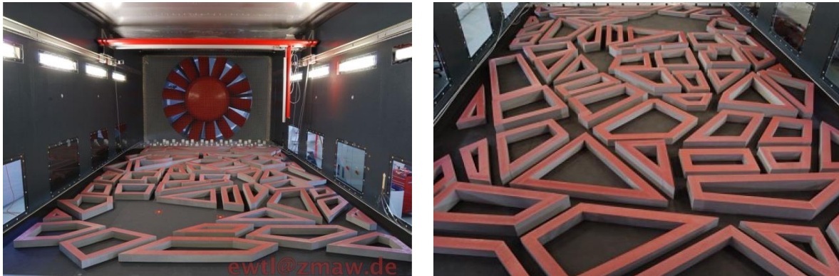
Fig. 1: The semi-idealized urban geometry used in this study (picture courtesy of EWTl, Bernd Leitl – left picture is from a later setup that had roughness elements both before and after the city).
