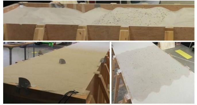
Fig. 3: Top- Preparation of the soil target. Lower right- The wetted 1m x 1m area at the location of the gravel-soil mixture. Lower left- The positioning of the reference trihedrals. Darkening of soil surface in vicinity of surface reference trihedrals is caused by shadow.
