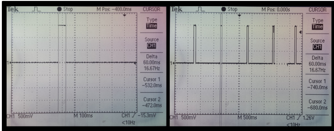
Figure 4.17.: Oscilloscope recording of circuit voltage modulated by servo impact. Circuit 'on' time measured by the oscilloscope to be 60ms: this is the total time that the circuit remains closed. This is equal to the total time it takes the PC to register the impact of the servomotor with the circuit and to send a signal back to retract the servomotor. Left: single impact, as recorded on the oscilloscope. The voltage rises sharp from 0V to 1.5V when the servomotor closes the circuit. Right: Multiple hits recorded over a 5s period.
