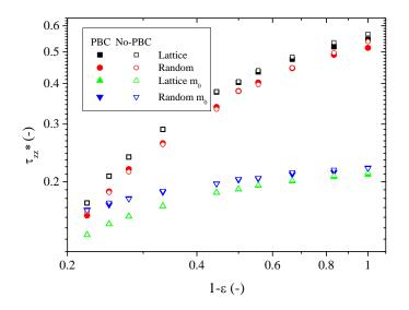
**Figure 6.-** Characterizing field-induced structuration process of MR fluids in quiescent state: a) magnetic energy, b) normal stress and c) average nearest neighbors per particle.
