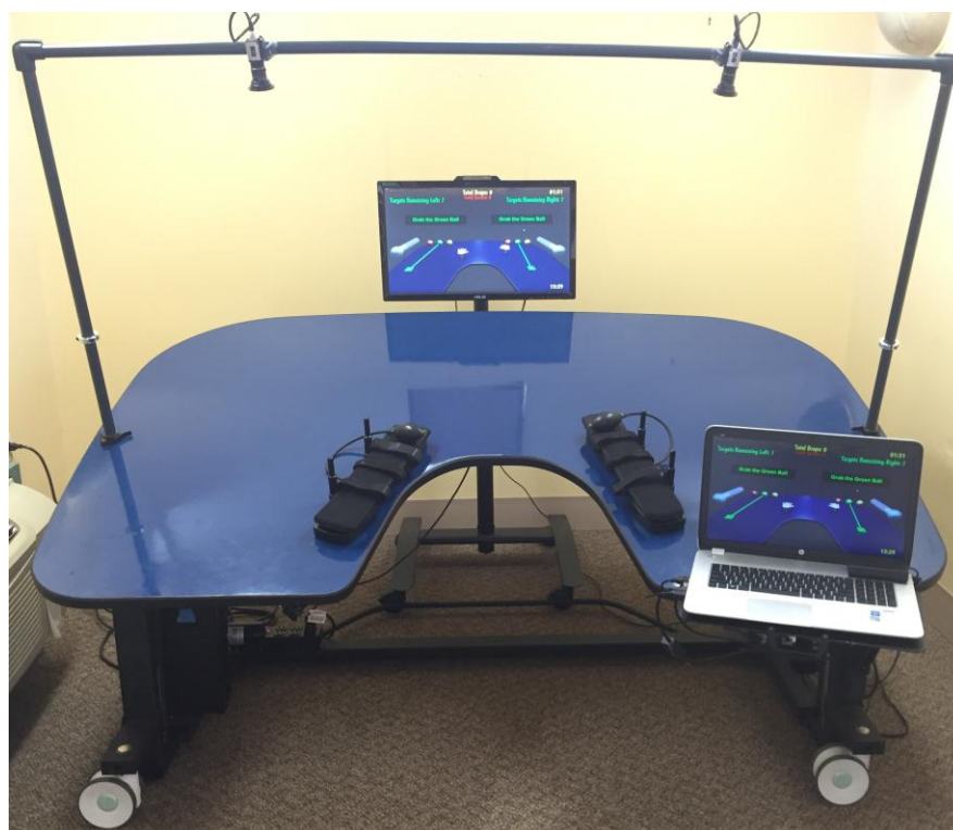
Figure 1. BrightArm Duo Table tilted upwards with two arm supports for user interaction and therapist laptop rendering Pick & Place game to the 27" monitor. © Bright Cloud International Corp. Reprinted by permission.
