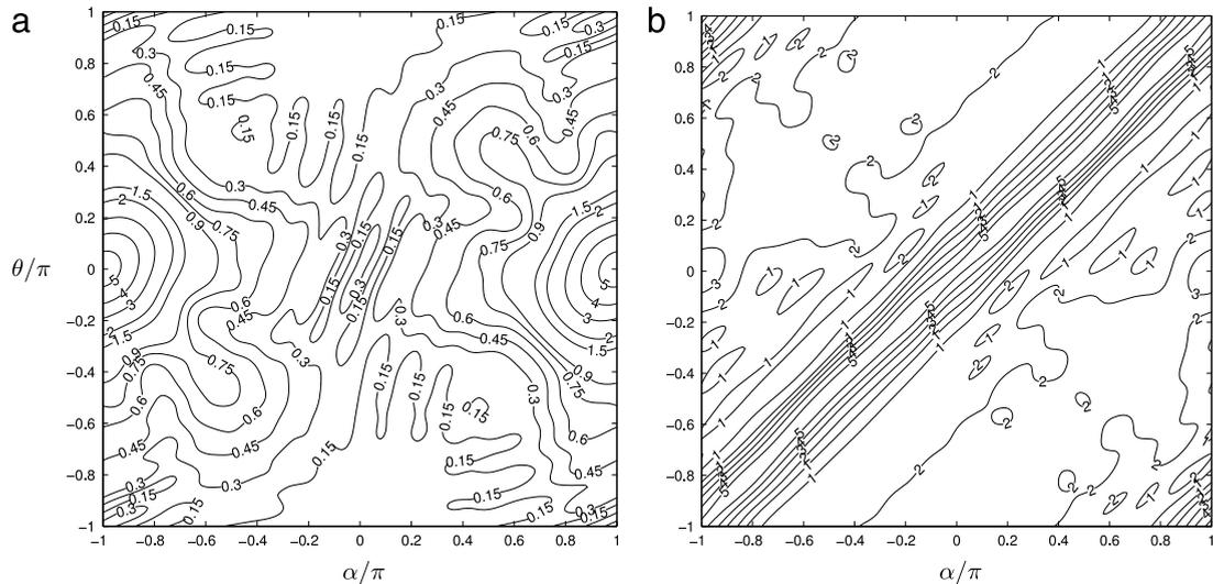
**Fig. 2.** Absolute value of far-field diffraction coefficients, for  $ka = 2\pi$  and  $\theta_1 = \pi/5$ , as functions of incident angle  $\alpha$  and observation angle  $\theta$ . Panels (a) and (b) display  $|F_g(\theta, \alpha)|$  and  $|F_g(\theta, \alpha) + F_c(\theta, \alpha)|$  respectively.
