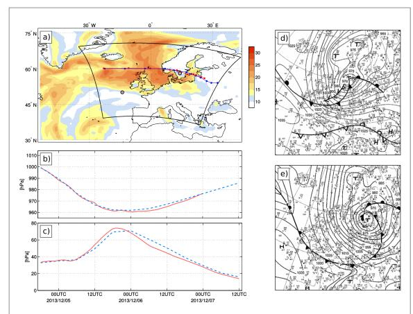
Figure 3. (a) Mean 10 m wind (in m s $^{-1}$ ) averaged over the simulation period 04/12 18 UTC-07/12 12 UTC. Xaver track as modelled by CCLM (red) and from ERA-Interim (blue) with six-hourly time steps (dots). (b) Change of pressure gradient between the two marked points (black circles with the red point in the middle) in (a). (c) Changes of core pressure over time. (d) Weather chart German weather service 05/12 12 UTC (e) same as d for 06/12 00 UTC.
