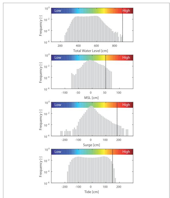
**Figure 5.** Histograms of each sea level component at Norderney over the observational record from 1999 to 2008. The black dotted line marks the magnitude during the high water peak of Xaver.
