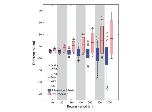
Figure 2. Differences between selected return water levels from the 1970–2013 minus 1970–2012 assessment from each grid point time series from the two-dimensional 'tide & surge' model separated into the two geographical areas of Schleswig-Holstein (blue) and Lower Saxony (red).
