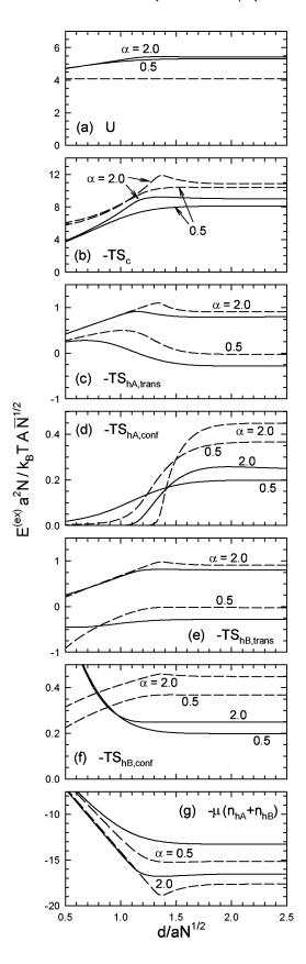
FIG. 7. The individual contributions to  $F^{(\mathrm{ex})}$  defined in Eqs. (18) and (25) as a function of monolayer spacing, d, calculated at  $\chi N = 100$  for two different molecular weight ratios,  $\alpha$ . (Note that  $\bar{N} \equiv \rho_0^2 a^6 N$ .) The solid and dashed curves denote the SCFT and SST results, respectively.
