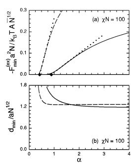
FIG. 4. (a) Depth,  $-F_{\min}^{(\rm ex)}$ , and (b) position,  $d_{\min}$ , of the attractive well as a function of the molecular weight ratio,  $\alpha$ , calculated at  $\chi N = 100$ . (Note that  $\bar{N} = \rho_0^2 a^6 N$ .) Solid and dashed curves denote SCFT and SST results, respectively. The tangent construction in (a) is used to indicate the point where the attractive well becomes negligible.
