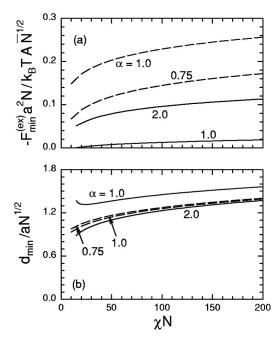
FIG. 3. (a) Depth,  $-F_{\min}^{(ex)}$ , and (b) position,  $d_{\min}$ , of the attractive well as a function of segregation,  $\chi N$ , for several molecular weight ratios,  $\alpha$ . (Note that  $\bar{N} \! \equiv \! \rho_0^2 a^6 N$ .) Solid and dashed curves denote SCFT and SST results, respectively.
