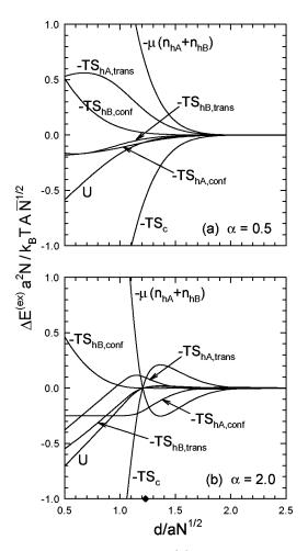
FIG. 8. The individual contributions to  $F^{(\mathrm{ex})}$  plotted together as a function of spacing, d, calculated using SCFT at  $\chi N=100$  for (a)  $\alpha=0.5$  and (b)  $\alpha=2.0$ . (Note that  $\bar{N}\equiv\rho_0^2a^6N$ .) So as to compare the relative importance of these contributions, each curve is shifted vertically so that it becomes zero at large d. In (b), a solid diamond indicates the position,  $d_{\min}$ , of the attractive well.
