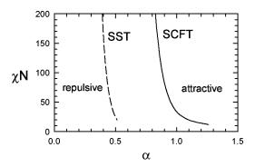
FIG. 5. Diagram separating parameter space (i.e.,  $\chi N$  and  $\alpha$ ) into regions where the monolayer interaction has a significant "attractive" well and where the interaction is essentially "repulsive." The criterion used to separate these regions is demonstrated in Fig. 4(a). The solid and dashed curves denote SCFT and SST predictions, respectively.
