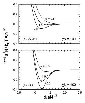
FIG. 2. Excess interfacial free energy,  $F^{(\mathrm{ex})}$ , as a function of separation, d, calculated at  $\chi N = 100$  for several molecular weight ratios,  $\alpha$ , using (a) SCFT and (b) SST. (Note that  $\bar{N} \equiv \rho_0^2 a^6 N$  is the invariant polymerization index of the diblock copolymer.) The solid dots denote the position,  $d_{\min}$ , of minimum energy,  $F_{\min}^{(\mathrm{ex})}$ , for those curves displaying an attractive well.
