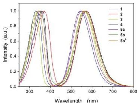
Fig. 7 Normalized excitation spectra (250-450 nm, excitation at the emission maximum) and emission spectra (400-800 nm,  $\lambda_{exc}$  = 350 nm). All measurements were done on powders at room temperature.
