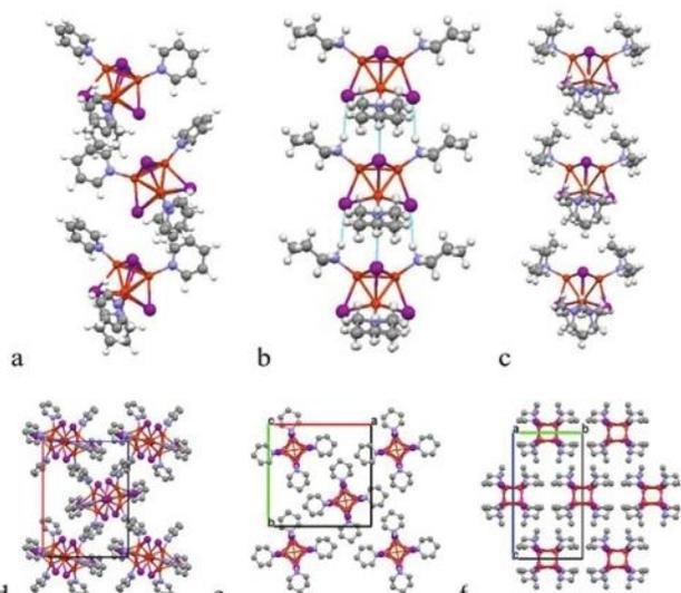
Fig. 2 The columns of cubane moieties in compounds 1 (a), 2 (b) and 3 (c) and how they pack in the crystal structures 1 (d), 2 (e) and 3 (f). In 2 (b) the N-H...I hydrogen bonds are highlighted in blue. In d, e, f, hydrogen atoms are omitted for the sake of clarity.
