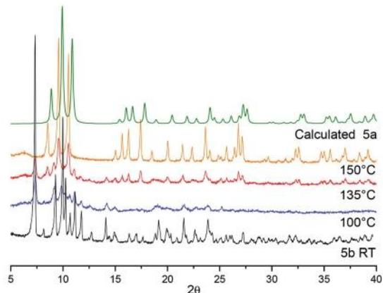
Fig. 6 Variable temperature XRPD analysis performed on **5b**, 100 °C: loss of crystallinity due to the solvent release; 135 °C (blue line): appearance of the **5a** phase at 135 °C (red line) and complete conversion to form **5a** at 150 °C (orange line). The green line is the calculated pattern of **5a** based on the structure solved at RT. The peak's shift of the orange pattern is ascribable to the cell expansion for the high temperature.
