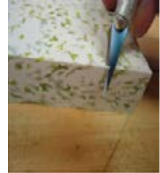
Figure 12a. Hardness test
