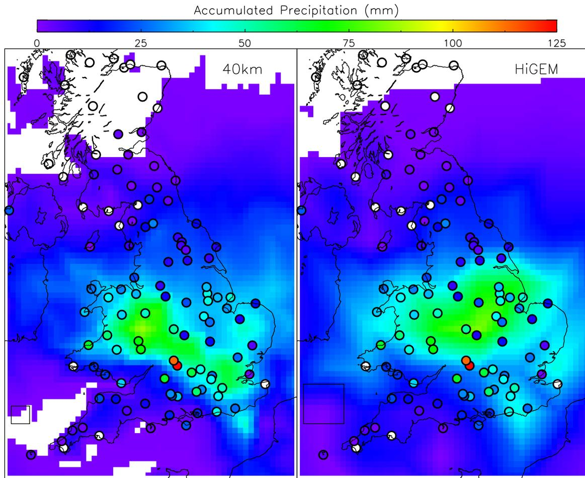
**Figure 4.** Comparison of the MIDAS rain gauges to the accumulated global (left) and HiGEM (right) model precipitation from 1200 on 19<sup>th</sup> to 0900 on 21<sup>st</sup>. The model data have been interpolated onto the 12 km LAM grid and the size of the original gridboxes is indicated.
