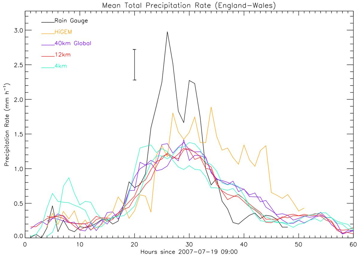
**Figure 1.** Hourly-mean precipitation rate averaged over a box representing England-Wales ( $4.5^{\circ}\text{W}$ – $0.7^{\circ}\text{E}$ ,  $50.6^{\circ}$ – $54.5^{\circ}\text{N}$ ) comparing model simulations with a rain gauge estimate. Both the model runs are plotted for the Global, 12 km and 4 km NWP configurations that used initial conditions at 0900 and 1200 UTC on 19 July 2007. The mean uncertainty estimated for the rain gauge observations on 20 July 2007 is indicated by the bar.
