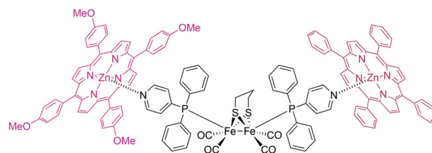
Fig. 1 The active [FeFe]H 2 ase biomimetic supramolecular assembly formed under photoreductive conditions from complex 1 in the presence of two different porphyrins.
