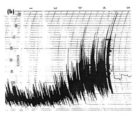
**Figure 8.** Wind-speed traces from anemometers at (a) Shoreham Airport (50°50′N, 0°17′W) and (b) Headcorn Aerodrome, Ashford (Kent), before they were broken by severe gusts at 0400 UTC and 0434 UTC, respectively. There is a zero shift such that the speeds in (a) are 4 knots too high.
