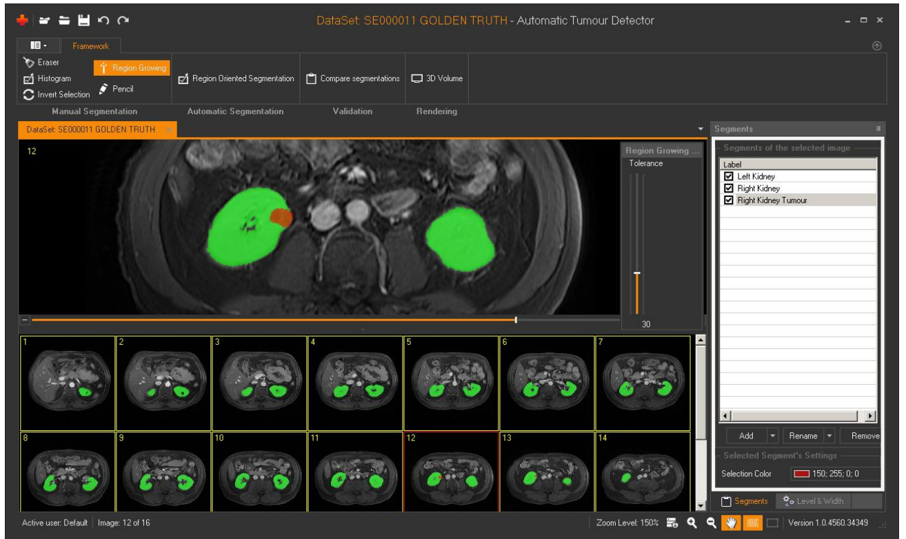
Fig. 2.1: Platform Design. The clinician has finished the segmentation task on slide no. 12. The Segments panel on the right side contains the delineated regions of interest (Left Kidney, Right Kidney and Right Kidney Tumour)
