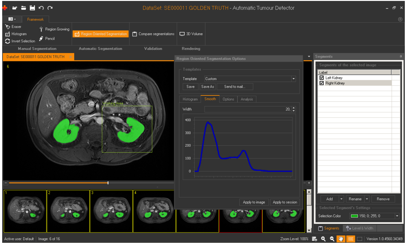
Fig. 3.3: Defining parameters and rules (“Templates”) for the Automatic Segmentation process
