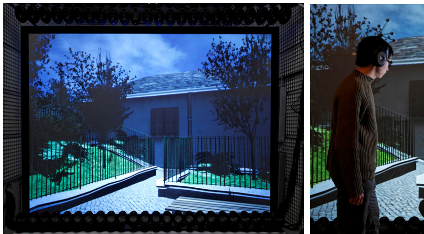
Figure 2. Virtual Reality setup. On the left, view of the entire screen in the acoustically damped studio, on the right, a participant equipped with headphones, a head tracker and polarized glasses.
