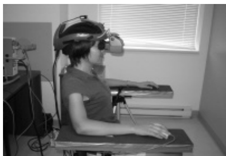
Figure 2. Experimental set up. Note position of contact thermode for QST under forearm, computer mouse controls temperature changes.
