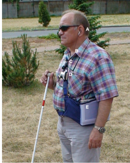
Figure 1. Trial participant wearing the prototype for communication with a remote assistant: A – earphone, B – microphone, C – Bluetooth GPS receiver, D – webcam with a fish-eye lens, E – Flybook laptop with built-in UMTS/HSDPA modem and touchscreen.
