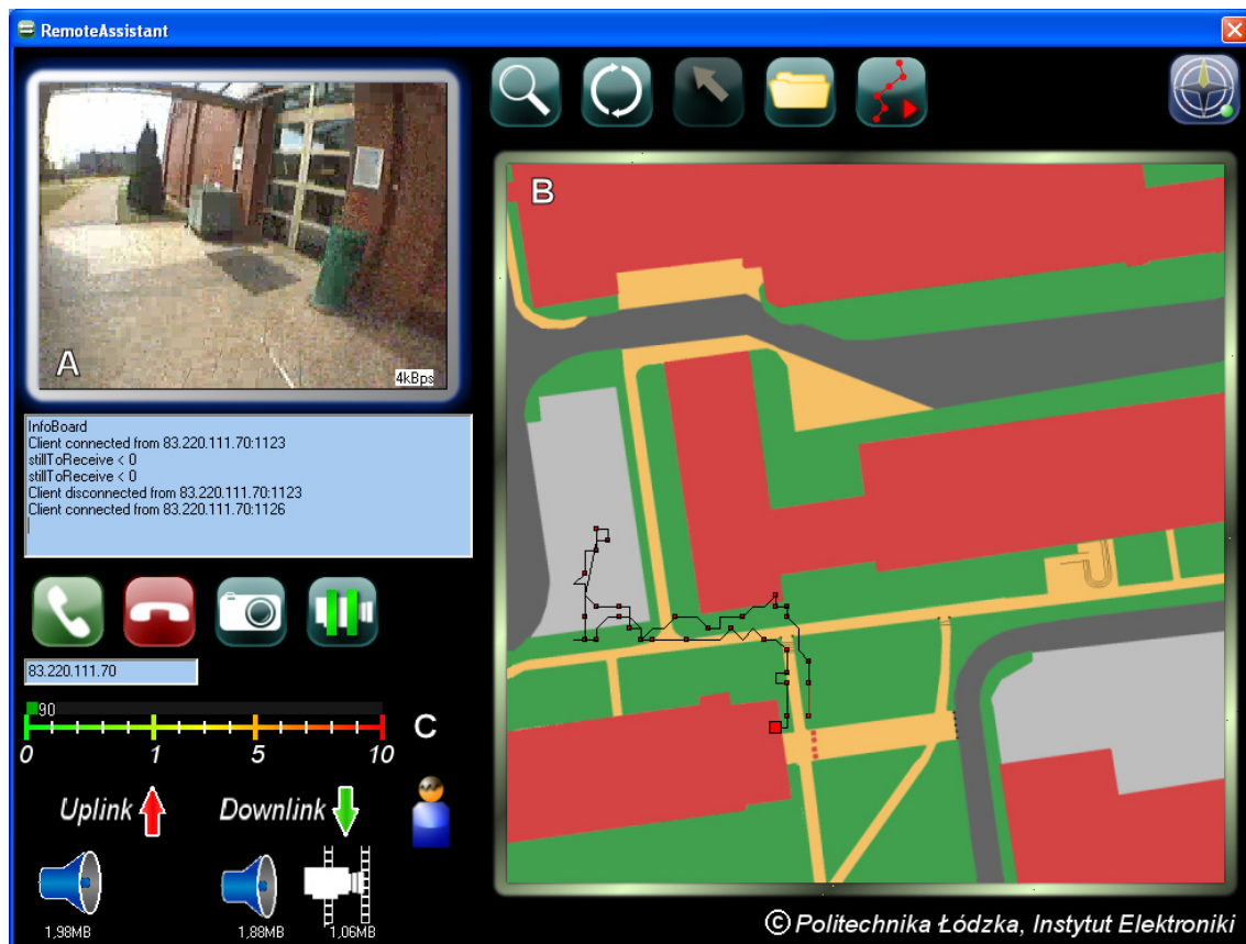
Figure 3. Screenshot of the operator's application: A) The video stream, B) Digital map with GPS readouts, with small markers every 5 seconds, C) Connection controls and parameters.
