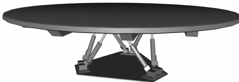
Figure 1. The CAREN platform (MOTek, Amsterdam, The Netherlands) can generate targeted movement perturbations which can be used to control game difficulty.
