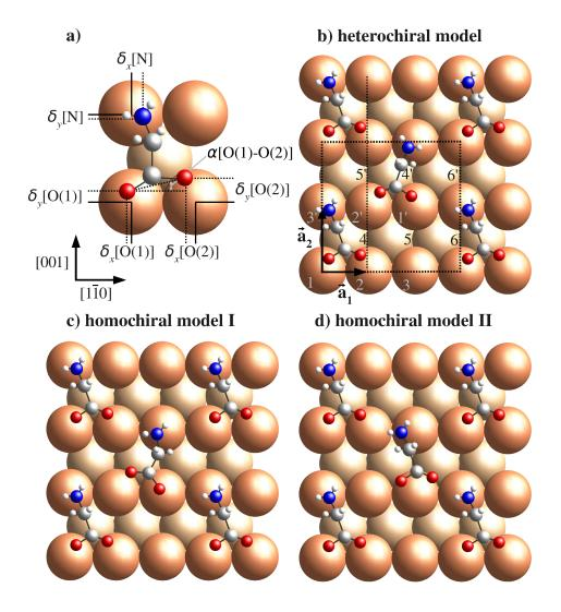
Figure 1: Schematic drawings of the model structures of glycinate overlayers on Cu{110}: a) a plan view of the best-fit structure; some of the structural parameters used in Table 2 are indicated; b) heterochiral model, in which the unit cell has a glide-line, indicated by the dotted line; c) homochiral model I suggested by DFT; <sup>15–17</sup> d) homochiral model II based on the structure proposed by Chen et al.; <sup>10</sup> models c) and d) do not have glide-line symmetry.
