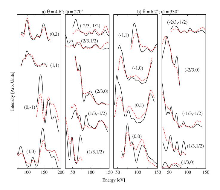
Figure 2: Selected representative experimental (black) and theoretical (red) LEED-IV curves for the best-fit structure of the heterochiral model.
