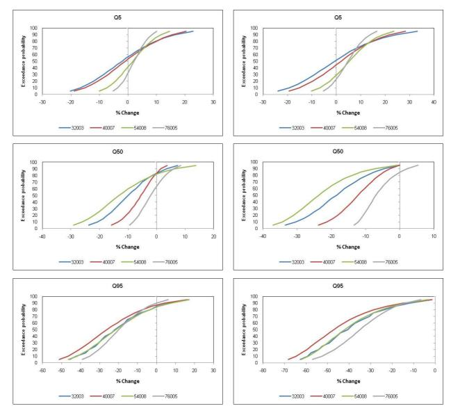
Figure 4.3 Probability distribution of change in flow statistics (Q5, Q50 and Q95) for the four sites for the 2020s and 2050s relative to baseline.
