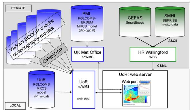
**Fig. 2.** Architecture of the system. Model data (blue) are ingested into the portal via an instance of ncWMS at the University of Reading (UoR), and an instance of ncWMS at the UK Met Office. in situ data (green) are ingested into the portal via the WFS at HR Wallingford serving CSML XML.
