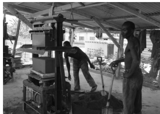
PLATE 2 A-sandcrete block just produced.
