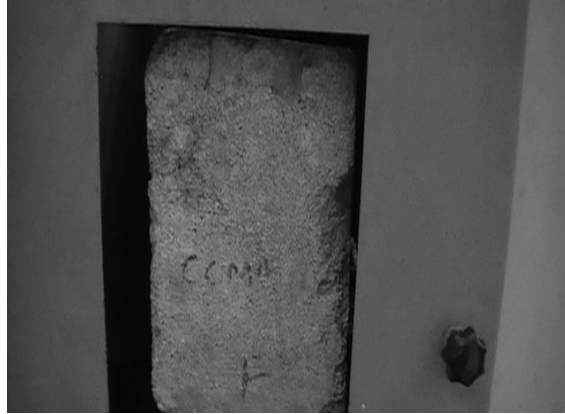
PLATE 4 Crushing test of one the sandcrete blocks.
