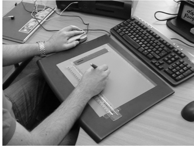
Figure 3. The user browses the graph using the graphics tablet for input with the dominant hand, and the VTPlayer tactile mouse for output with the non-dominant hand.
