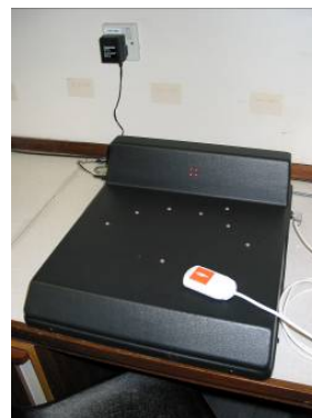
Figure 2. The Piercy Adams Choice Reaction Timer.
