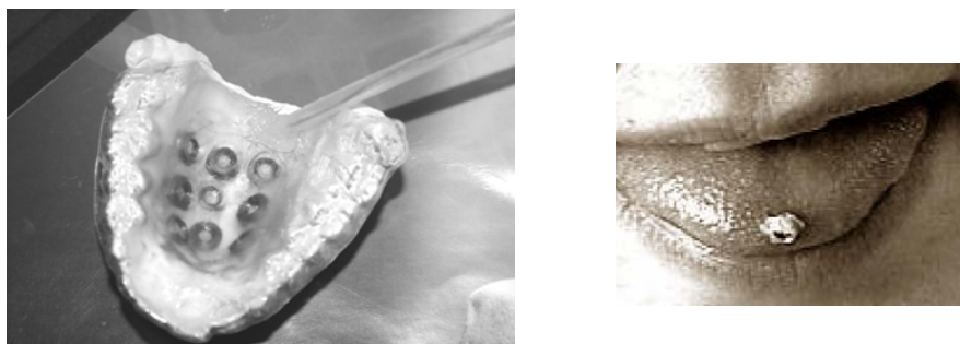
Figure 2. Left: The palatal plate (placed on a mould of the upper part of the mouth) with inductive coils and a silicone tube leading the wires out of the mouth. Right: The activation unit glued to the tongue.
