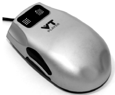
Figure 2. The VTPlayer tactile mouse ( www.virtouch2.com ). The mouse incorporates two, 4-by-4 tactile pin-arrays, on which the index and middle fingers are placed during operation.
