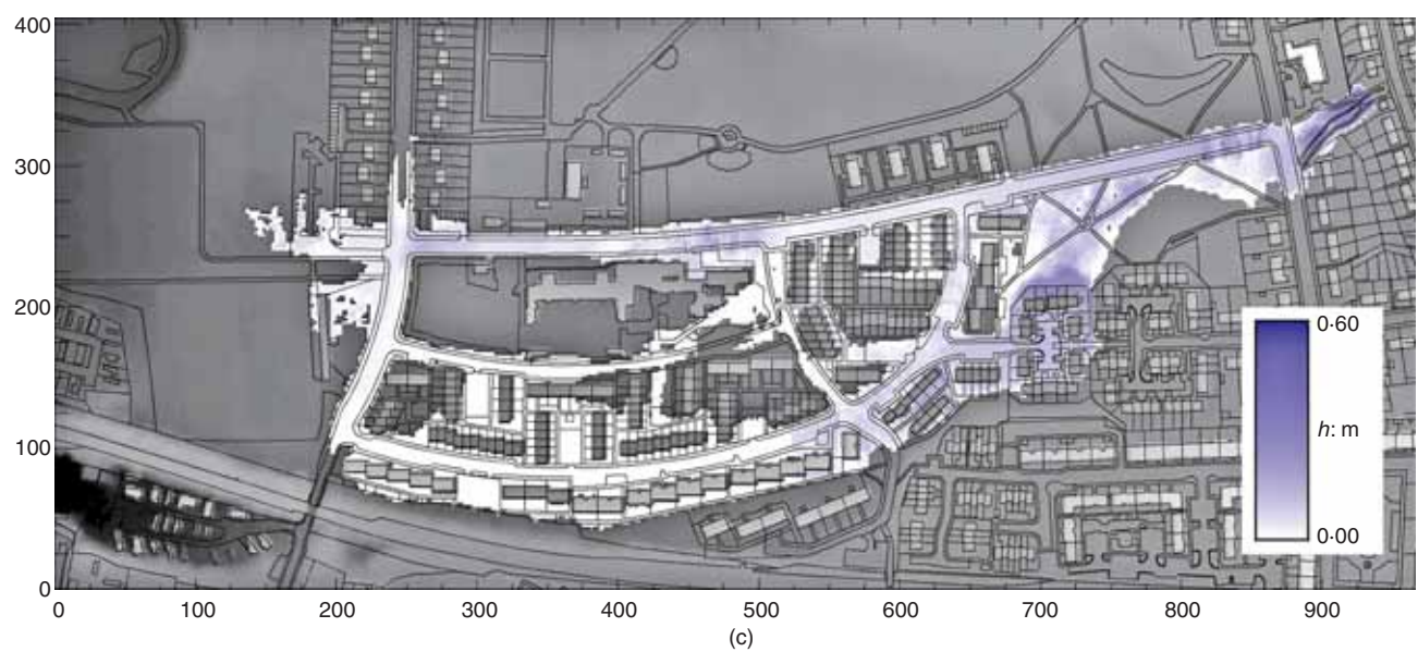
Fig. 8. Magnitude of range in maximum predicted water depth ( h ) in each model grid cell over the whole event for the ensemble of varying friction coefficient simulations shown in Table 2: (a) DIVAST; (b) DIVAST-TD; (c) JFLOW; (d) LISFLOOD; (e) TRENT; and (f) TUFLOW
