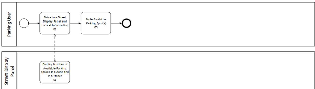
The city maintains several street display panels that show the available number of parking spaces in nearby parking zones and streets (Step 01). This enables the driver to quickly determine, while driving, where it would be most likely to find an available parking space and to direct the car to the street (Steps 02 and 03). The functionality of the system (M) thus enables the driver (H) to modify his or her behaviour:
