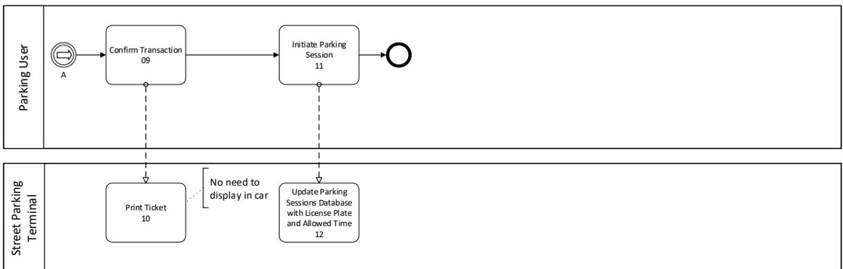
After confirming the transaction (Step 09), the ticket is printed (Step 10), and the parking session initiates (Steps 11 and 12). In case the person selected payment via credit card, the process flow branches off as follows:
