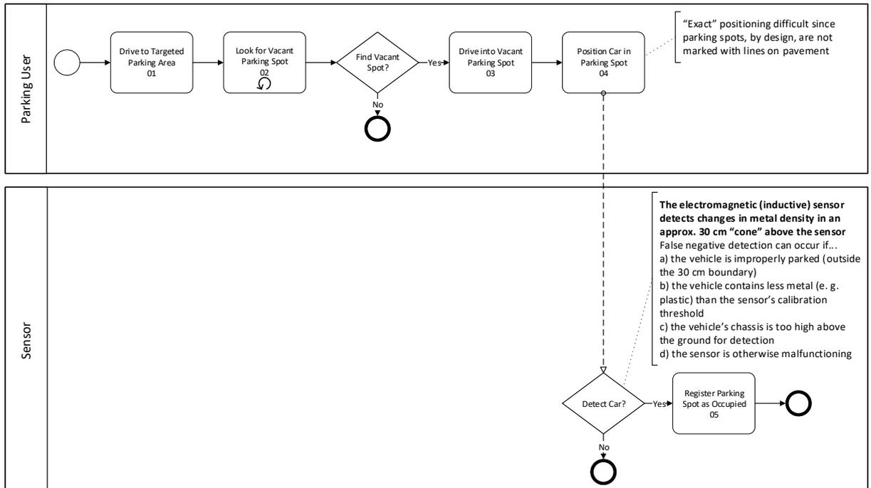
The user selects a parking spot (Steps 01 and 02), enters the spot (Step 03), and parks the car (Step 04). At this point, the system marks the parking spot as 'occupied' (Step 05). The human action of parking the car (circle H) prompts for the sensor (circle M) to pick up the car's metal density:
