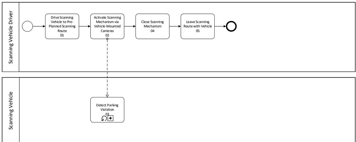
After positioning the vehicle at the start of the scanning area (Step 01), scanning takes place (Step 02). Process 12 handles the detection of parking violations. At the end, Process 11 completes by closing out the session in Steps 04 and 05.
