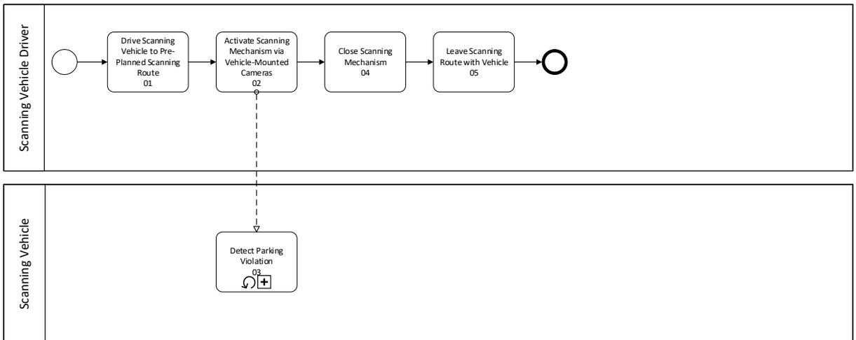
Step 01 positions the vehicle at the start of the area to be scanned whereby the actual scanning occurs in Step 02. Parking violations are then detected by the system (Step 03 – further explained in Process 12 below) and the scanning session is closed out Steps 04 and 05.
