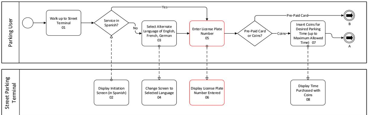
The process is laid out where the person walks up to the terminal (Step 01), makes the appropriate selections on the screen (Steps 02, 04-06) and submits payment (Step 07), where then the parking time is displayed (Step 08).
