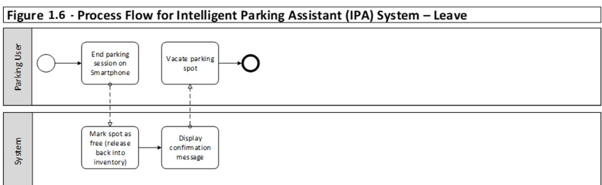
After ending the parking session on the smartphone, the system releases the occupied parking spot so that it shows as ‘available’ for other users. The driver then vacates the parking spot.
