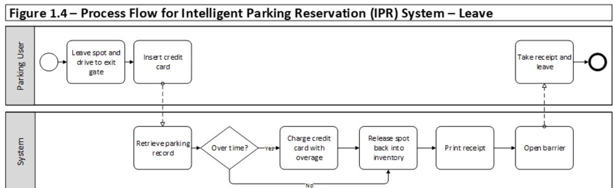
In this flow, the user drives with the car to the exit gate. After inserting the credit card into the reader, the system matches the corresponding parking session via the credit card information that was previously recorded when entering the car park. If the allowed time is exceeded, the credit card is charged with an overage fee. The parking spot is then released back into inventory, the receipt is printed, and the driver is free to leave the facility.
