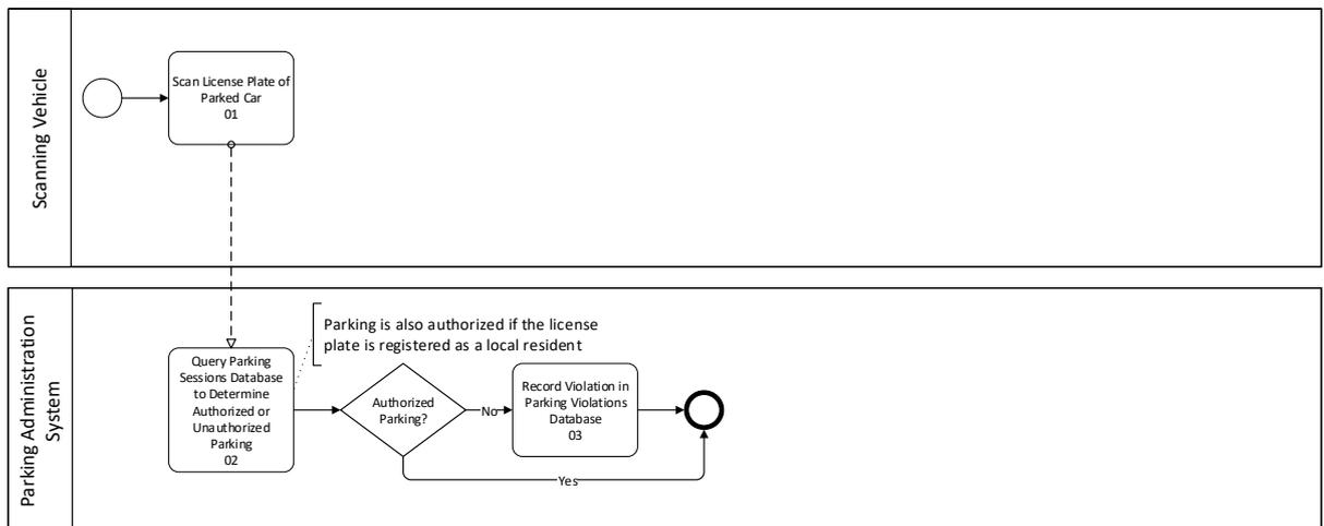
The system scans the license plate in Step 01 and queries the Parking Sessions Database to determine if parking for this license plate has been paid for (Step 02). If the license plate is determined as 'not authorized', the system records the violation in the Parking Violations Database (Step 03). The design (circle I) is comprised of largely automated processes that are executed within circle M:
