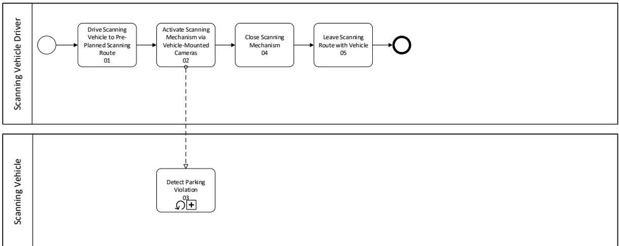
Initially, Step 01 positions the vehicle at the start of the area to be scanned whereby the actual scanning occurs in Step 02. Parking violations are then detected by the system (Step 03) and the scanning session is closed out in Steps 04 and 05. The system is designed to perform these steps most efficiently while continuously operating. The I → M pathway and the (human) scanning vehicle driver operates the device as intended as expressed through the H → M line:
