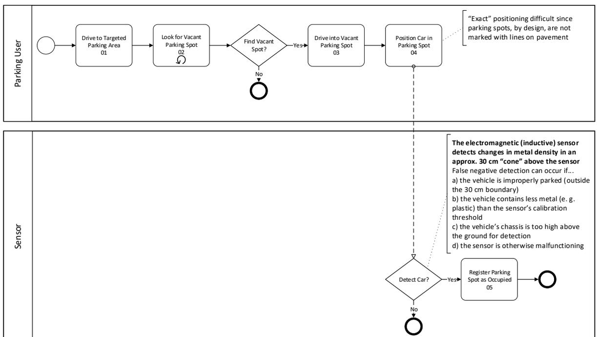
Once the driver selects and parks the car (Steps 01-04), the next process stage is for the sensor to detect the parked car, before the parking spot can be registered as 'occupied' in Step 05. The system is designed to confirm that a vehicle is above a parking sensor for the space to be registered as 'occupied'. From an SBF pathway perspective, the user parks the car on top of the sensor (H → M), which allows the sensor to recognize and record its current unavailability for other users:
