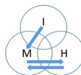
The design expects for the terminal to receive the license plate number as expressed in arrow I → M. Arrow M → H prompts the user to enter the license plate while arrow H → M then receives the entry.
