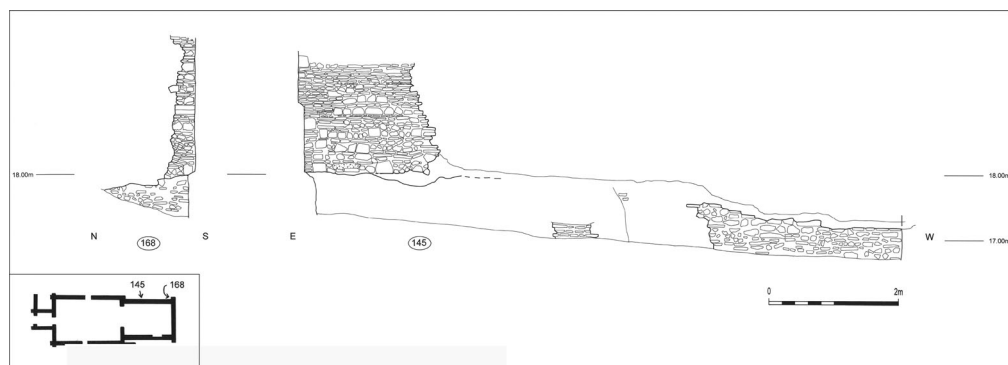
FIG. 8. St Pancras Chapel, north wall and north-east buttress (stipple indicates plaster base/render).
